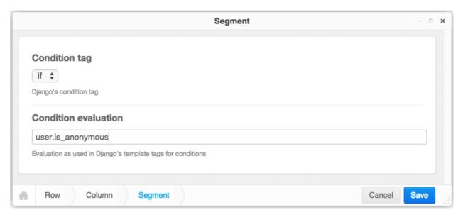
This plugin now behaves as an if block, which is rendered only, if the specified condition evaluates to true. The syntax used to specify the condition, is the same as used in the Django template language. Therefore it is possible to evaluate against more than one condition and combine them with and, or and not as described in boolean operators in the Django docs
