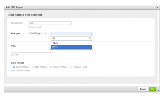
The behavior of this Plugin is what you expect from a Link editor. The field **Link Content** is the text displayed between the opening and closing <a> tag. If used in combination with djangocms-text-ckeditor the field automatically is filled out
